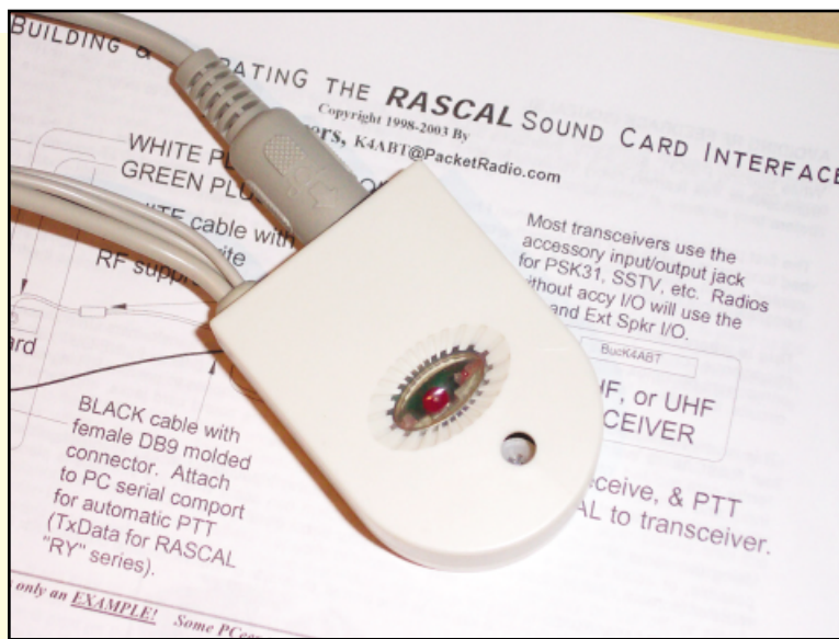
The K4ABT RASCAL sound-card interface. It is an inexpensive and relatively simple device, using good isolation transformers and ferrite beads to avoid feedback issues. Note the transmit audio level adjustment potentiometer inside the small hole. For more information, go to < www.packetradio.com >.
